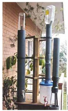
Figure 3. A granulated media water filter suitable for households costs \$3 to \$6.
